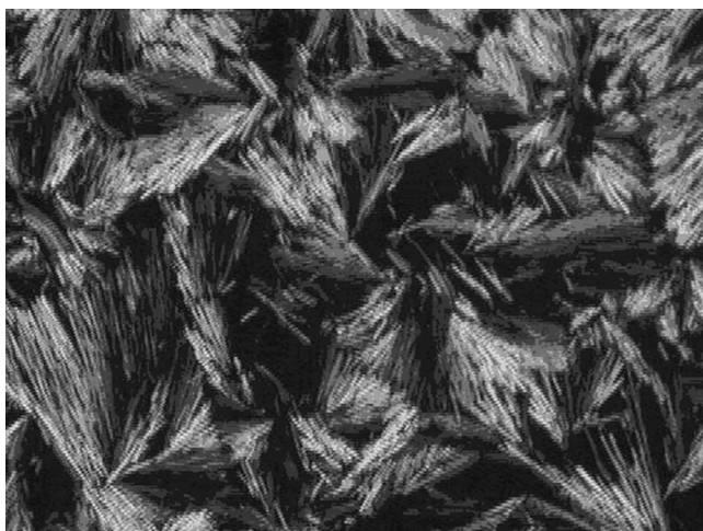
FIGURE 8 Filamentary texture of TGBA phase of CN. ( \times 100 ), 84°C.
