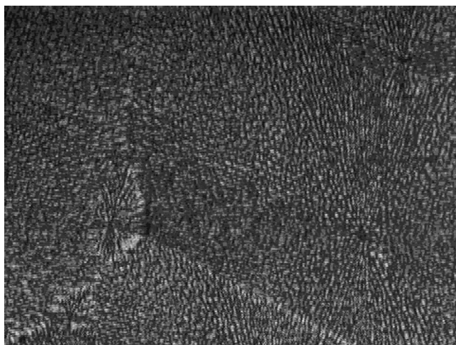
FIGURE 2 Texture of cholesteric phase of CN. ( \times 100 ), 80^\circ\text{C} .
